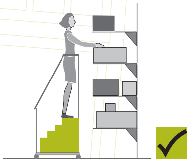
Figure 5.9 . Control the risk of storing things at height.
