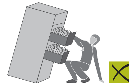
Figure 5.11 Filing cabinets may be unstable when fully loaded and the top two drawers are open
